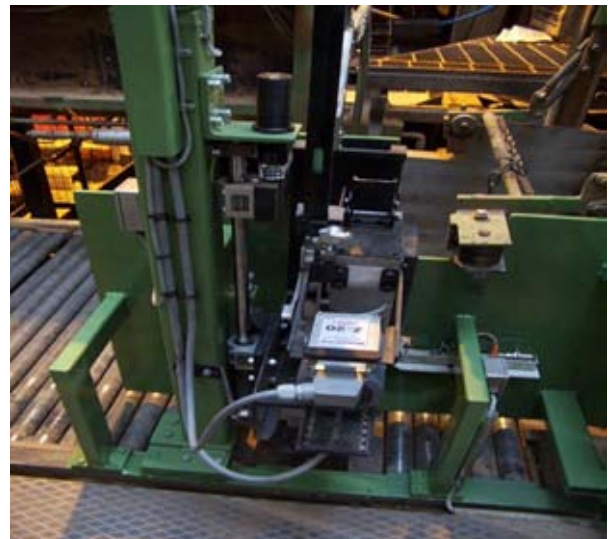
Simple slide-in-and-fix carriage for the sealer unit is easy to use as no tools are required
