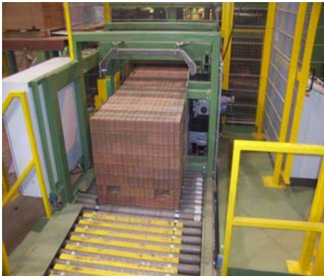
Easy access on tensioning modules to strap path for Maximum machine throuput in brick/paver machines
