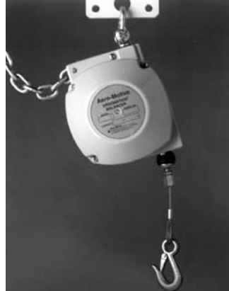
EB2500R Part No. 485001* 18-25 lbs. (8.2-11.4 kg), 6.6 ft. (2 m) cable travel
