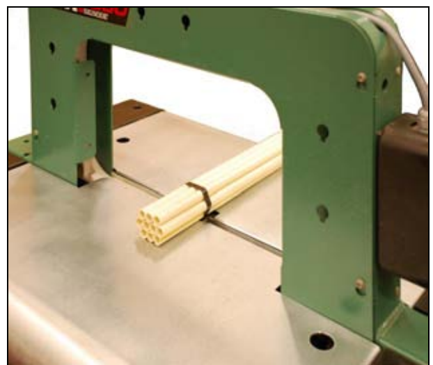
Small and round packs strapped with 9 mm PP
