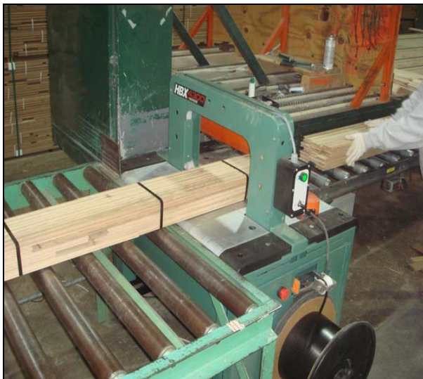
Suitable for solid lumber products as small as 70 x 20 mm
