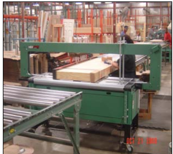
HBX 4300 large frame model integrated into flat-pack door packaging line (short anvil not available on this model)
