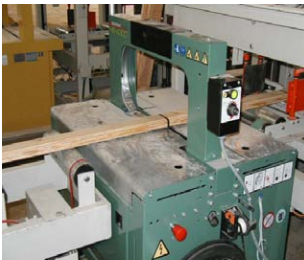
HBX 4300 machine inline strapping lumber millwork
