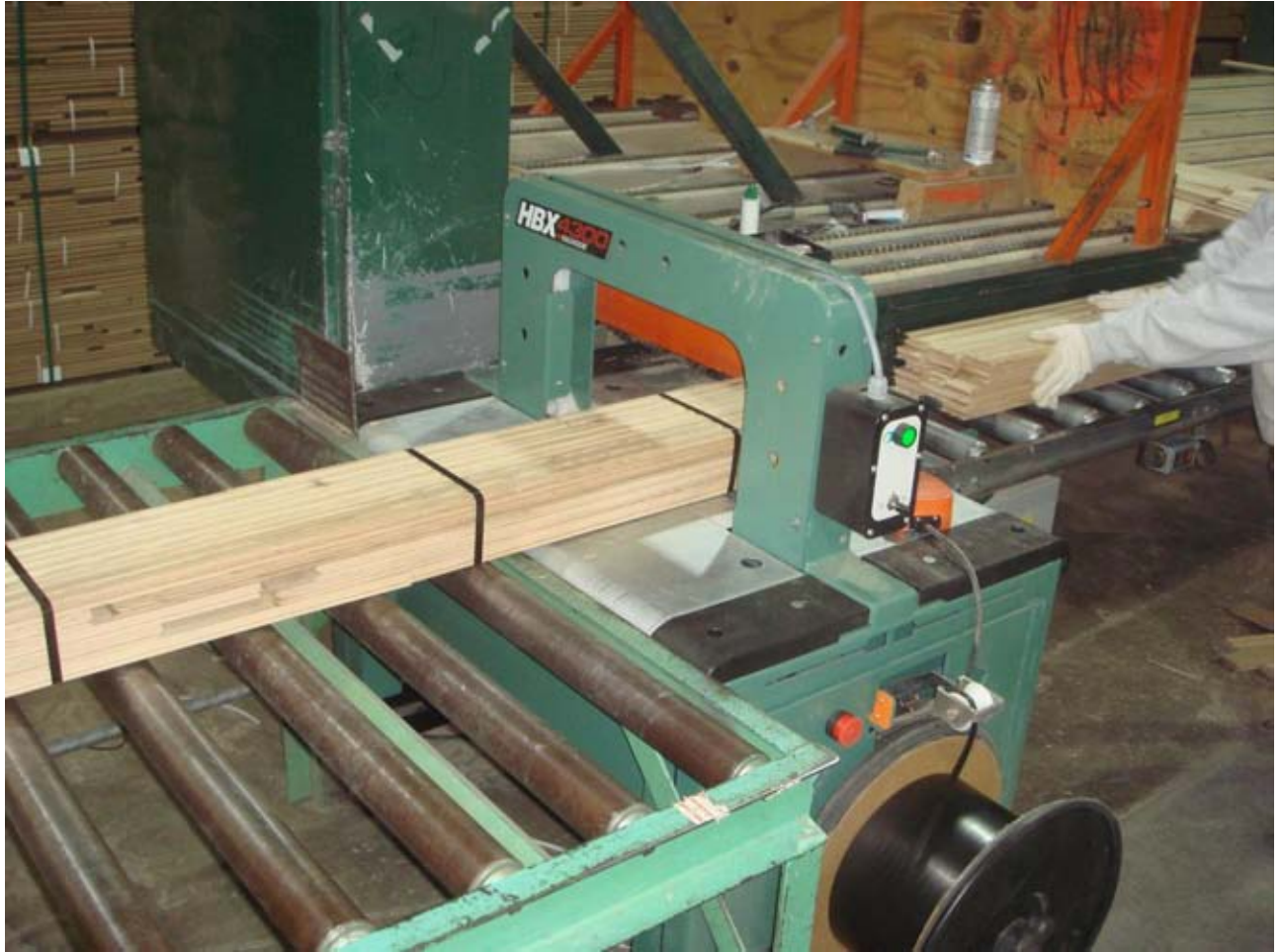
Securing wooden flooring with 9 mm PP plastic strapping with the HBX 4300 short anvil machine
