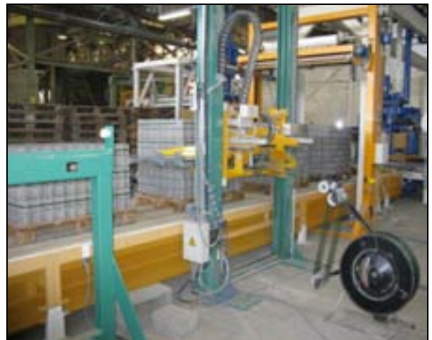
Modular MD-H horizontal strapping machine, with easy strap thread-up and the lowest TCO system available
