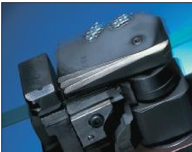
Swing-weld spare sealer module for maximum machine Uptime, easy to remove and re-install by removing four bolts
