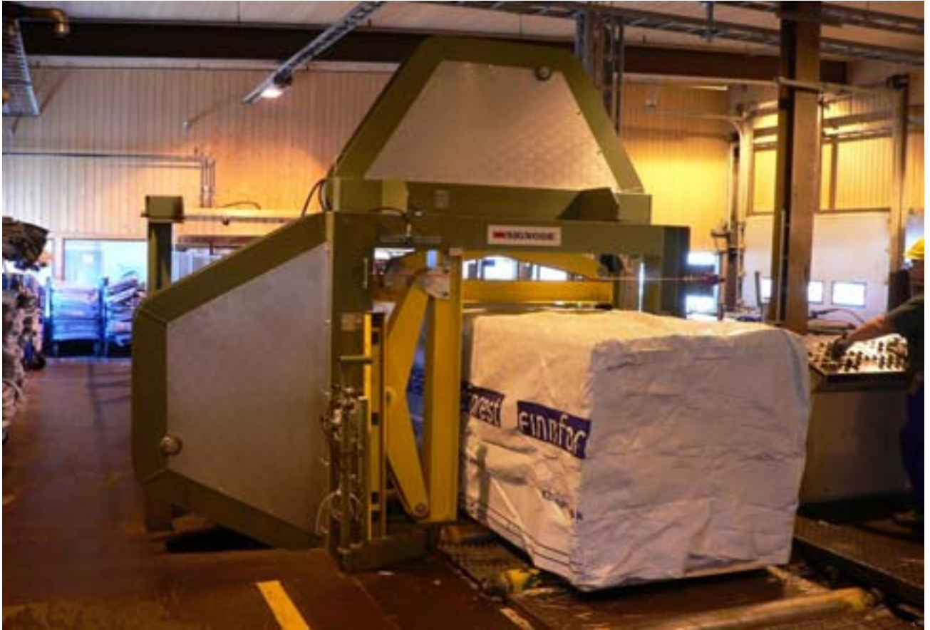
Model Z-20 press with top/side compression & squaring arms & side-mounted, moving Z-20 ® strapping head.
