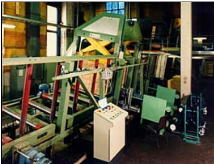
Model shown as HD-S-LP Tandem operation load compression and securement with PET strapping
