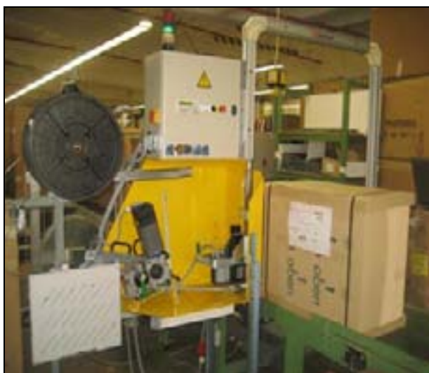
Fully automatic strapping of packaged kitchen cabinets
