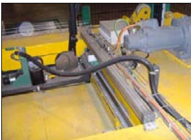
It is very easy to change the light-weight sealer module Seen here is the indexing sealer unit on a twin chute model
