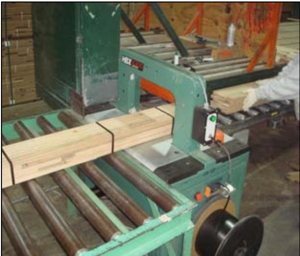
HBX 4300 machine strapping lumber millwork
