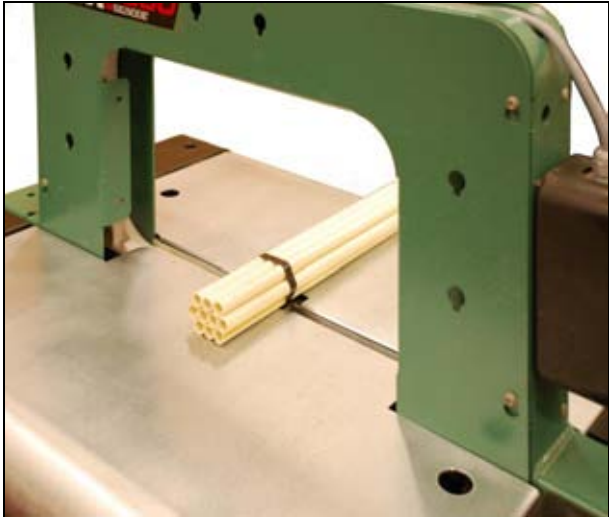
Small round packs strapped with 9mm PP strapping
