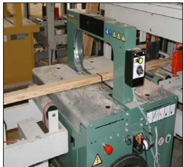
HBX 4300 integrated into automatic packing line
