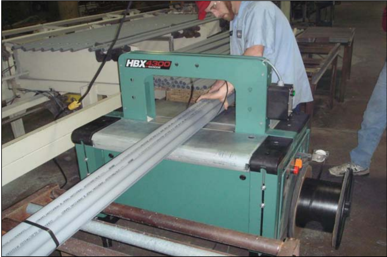
Securing plastic water pipes with 11 mm PP plastic strapping with the HBX 4300 short anvil machine
