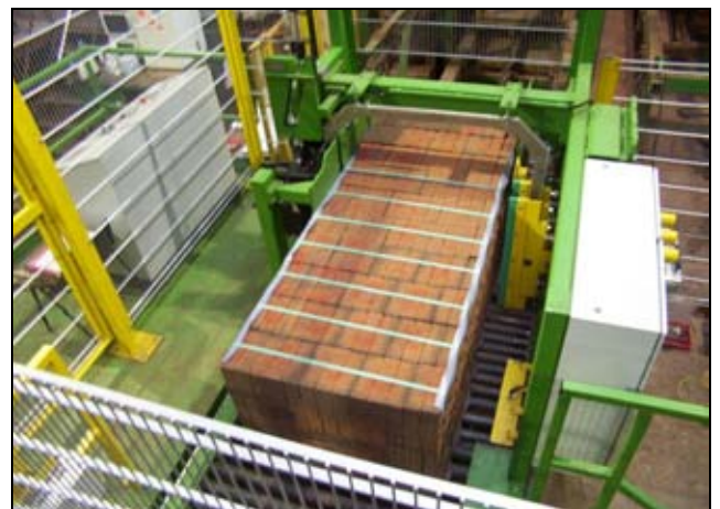
Packaged brick packs safely secured with Tenax ® PET high-strength 16 mm polyester strapping
