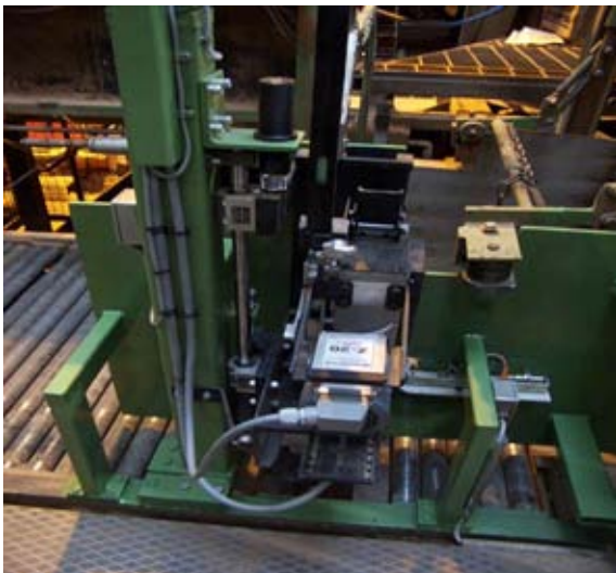
Side mounted strapping head, fully electrical in operation, can be removed easily for servicing
