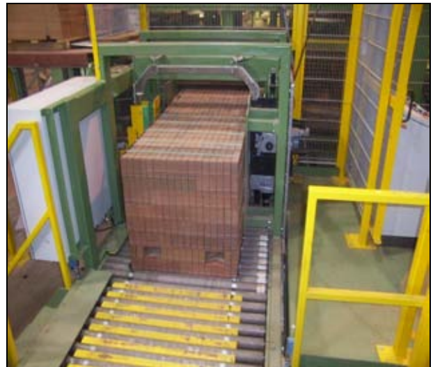
Compacted brick packs , secured with PET Tenax ® high-performance 16 mm polyester strapping
