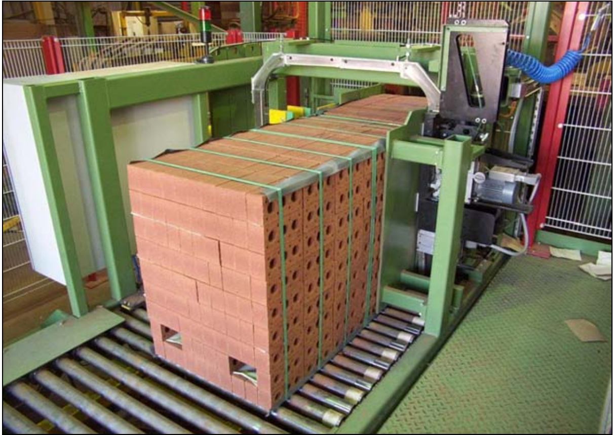
Signode Z-20 Brick Packaging station with integrated compactor arms, Z-20 strapping system, top edge protection applicator units for Bladerunner-Retrax materials, packaging high-quality facing bricks
