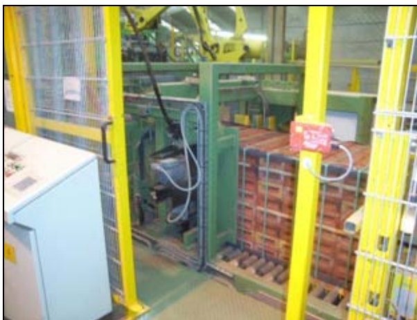
Easy access side mounted Z-20 head module, for high speed applications twin heads can be installed
